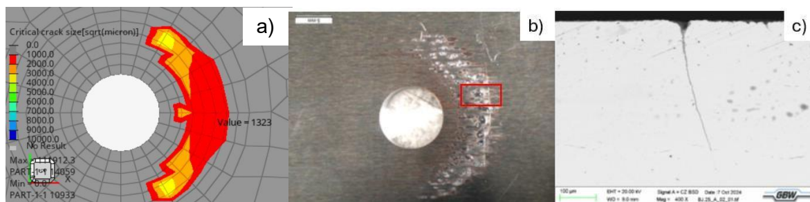
Figure 1: a) Simulated fretting damage area and critical crack size. b) Fretting scar in the experiment. c) Crack found from the fretting spot.
