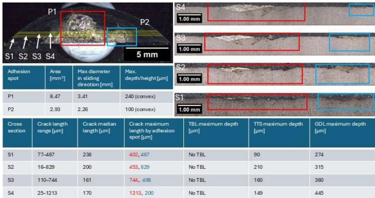
Figure 1: Characterization of cross sections from a gross sliding test (sliding amplitude = 50 μm, normal pressure = 30 MPa, loading frequency = 40 Hz, 10 000 loading cycles).
